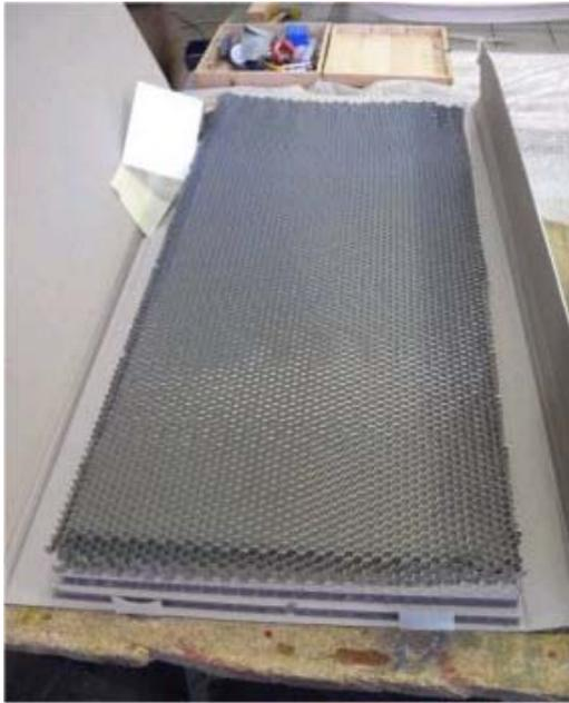
**Radiator :** The first trouble was with the radiator. The search for a suitable one resulted in a world wide quest. Finally the solution was in Belgium. Thanks to the Hexcel composites company, we can find the honeycomb structure needed to manufacture a fake radiator for the de Caters. The parts are now in the hands of Pascal to build this radiator
